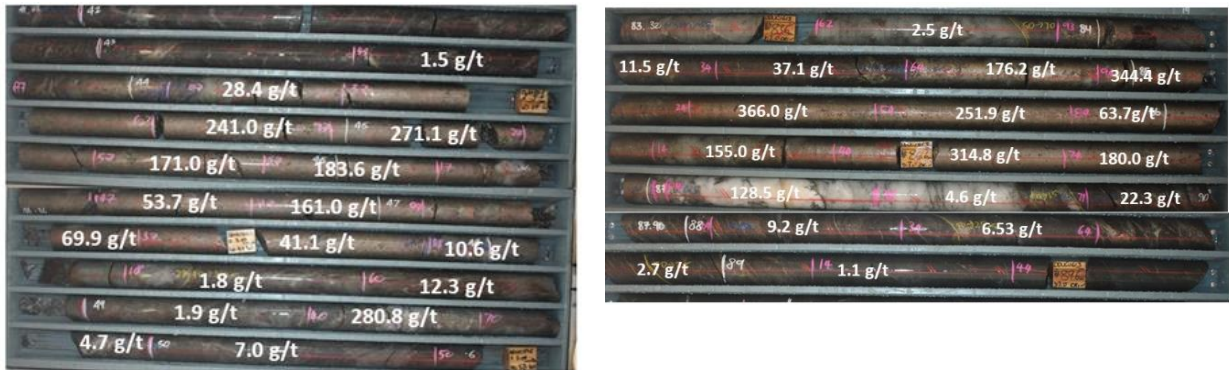
Figure 3: Left - DDUG1545 (10.8m @ 66.8 g/t gold) and Right - DDUG1613 (8.9m @ 71.1 g/t gold) showing massive pyrrhotite with milled quartz and abundant visible gold and consistent high-grade gold, this intersection is characteristic of the main shoot position recently defined in the upper southern levels of Deacon Main.
