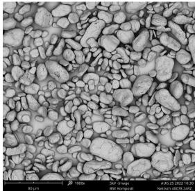
Figure 1. 99.99% carbon spherical graphite produced from Campoona concentrate (SEM image; 5kV, 1000x magnification, image ~ 320 microns across)
