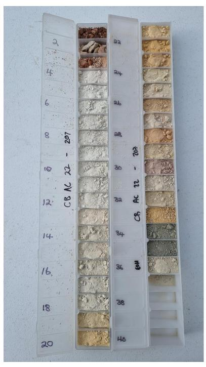
Figure 3. Chip tray of sample from drill hole CBAC22-207which contains 30m @ 1783 ppm TREO from 3m
