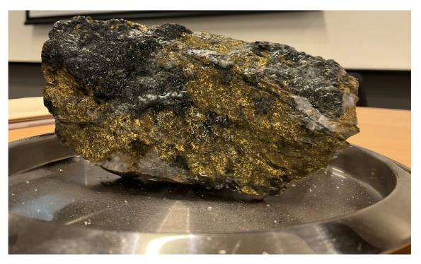
Figure 4 – Grab Sample from Nightfall Lode (visible gold evident).
