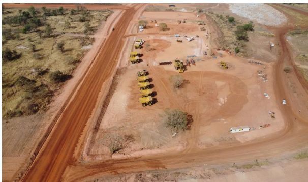
Image 5: Mining fleet – CAT777 trucks and CAT 6030 Excavator
