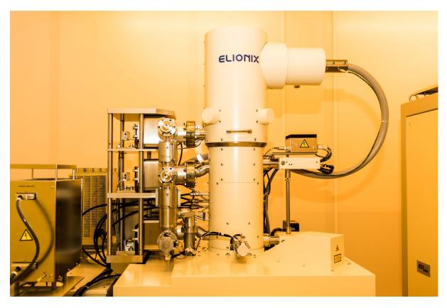
**Image 1. Elionix ELS-125 electron lithography system.** The vertical circular tower is where the electron-beam is located, while the chip is introduced through the load lock (the rectangular area with the protruding rod). The multi-million-dollar E-beam system is housed in a cleanroom environment in Sydney, Australia, and is manufactured in Japan.
