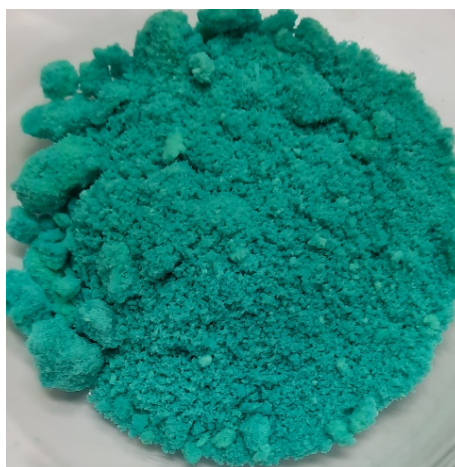
Figure 1: Nickel sulfate crystals produced from QPM pilot plant MHP
