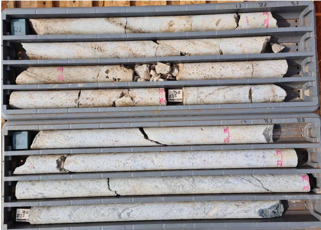
Figure 3 Carbonatite with stylolite joints and vugs. Fine grained disseminated rare earth minerals visible under hand lens. Low level of chlorite alteration from 77.10m onwards.
