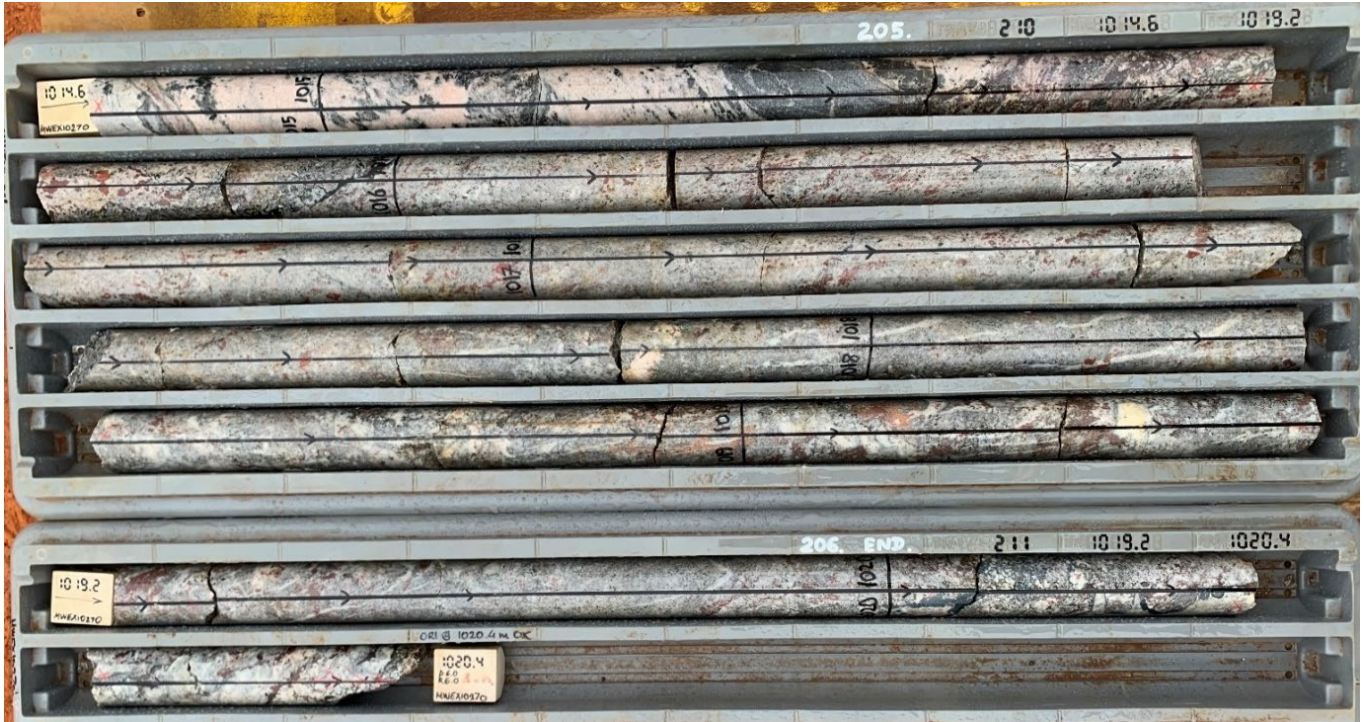
Figure 3 MWEX10270 Drillhole ending at 1020.4m depth in REE mineralisation
