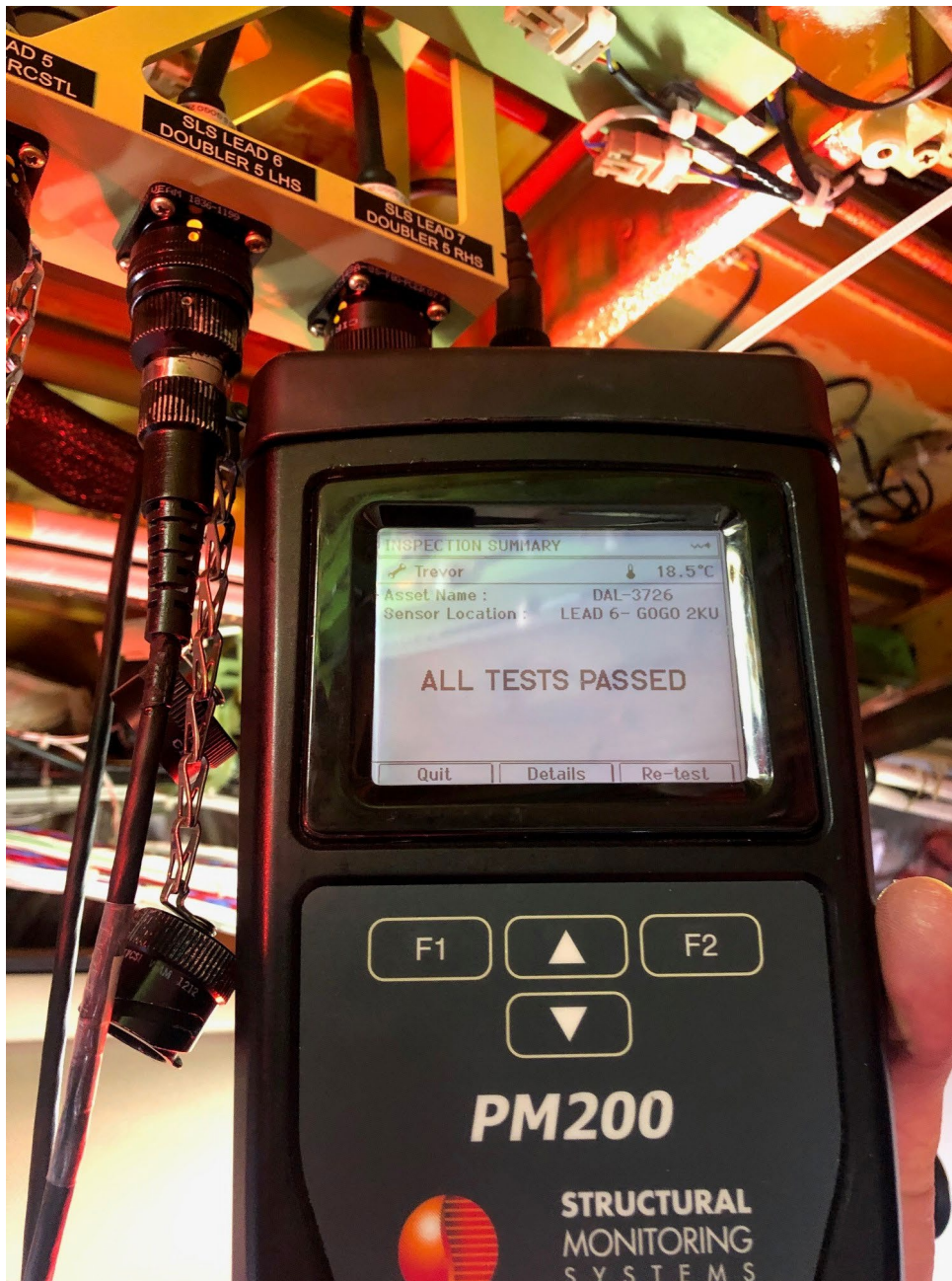
Figure 4. PM200 Test box indicating SLS Lead 6 (zone with approx.. 30 fasteners) Passed
